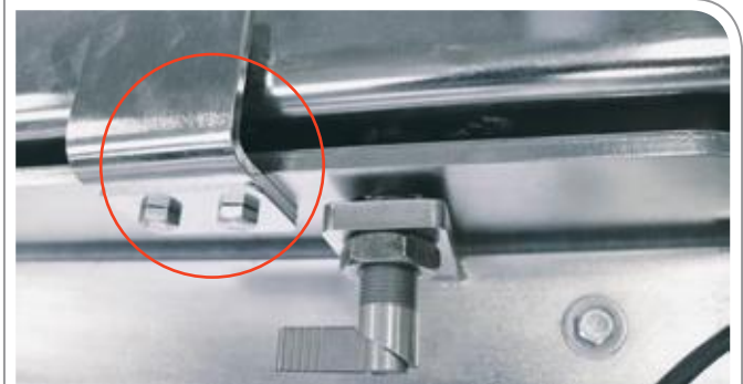
Screws, angles and spaces are susceptible to contamination and difficult to clean.
