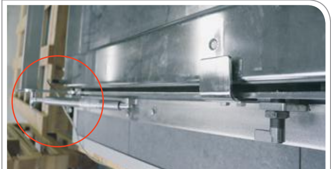
The externally mounted lift mechanism of the flat-bed scale requires additional space and represents a trip hazard for the operating personnel.
