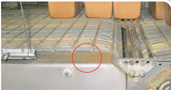
Horizontal deposit surfaces increase the effort required for cleaning
