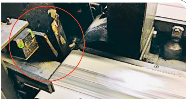
Large-scale deposits in areas which do not come into contact with the product mean less risk of contamination, but still necessitate increased cleaning effort.
