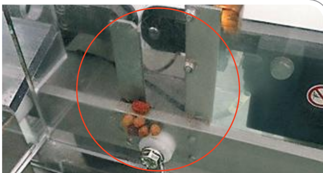
Deposits in difficult-to-access areas equate to effort in cleaning
