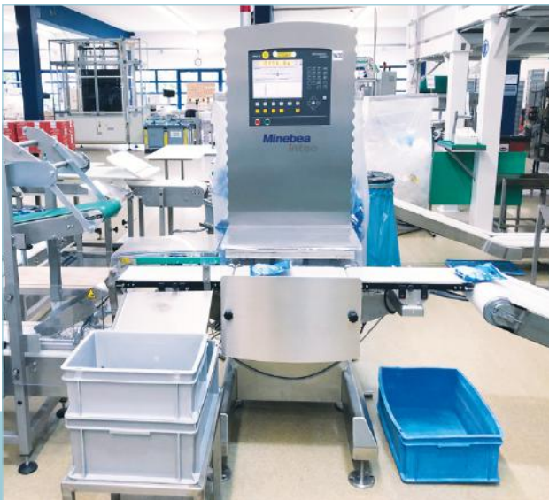
The checkweigher Synus guarantees reliable measuring results on the packaging line, thus contributing to product quality
