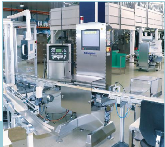
To start the batch, production-related data is entered to the checkweigher
